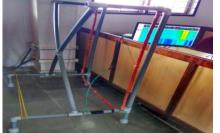
Figure.1.The VLF loop antenna and system running the spectrum lab software
